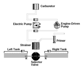
Figure A-1 Pressure-Feed System
