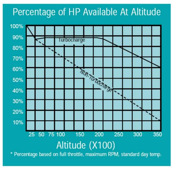
Figure A-1 Percentage of Horsepower Available at Altitude
