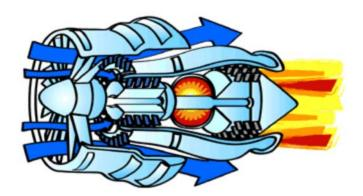
Figure A-3 Airflow Through a Turbofan Engine
