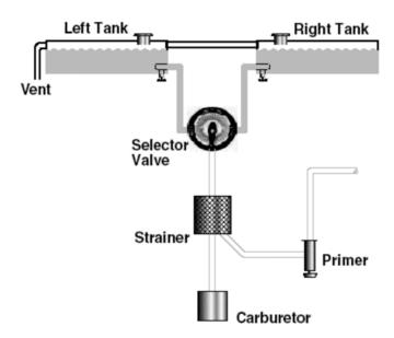
Figure A-2 Gravity-Feed System
