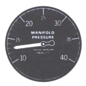
Figure A-4 Manifold Pressure Gauge
