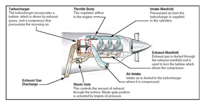
Figure A-2 Turbocharger Components
