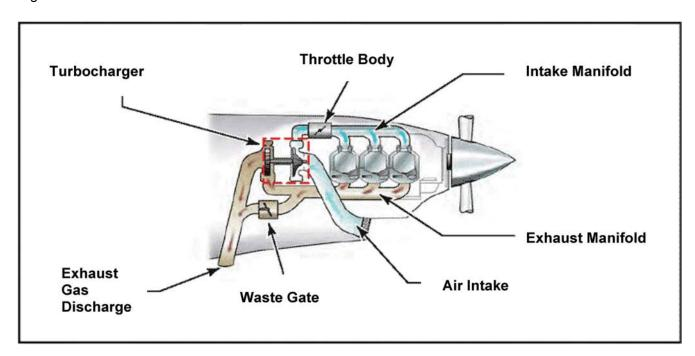
Figure C-1 Turbocharger Components
