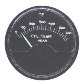
Figure A-2 Cylinder Head Temperature Gauge
