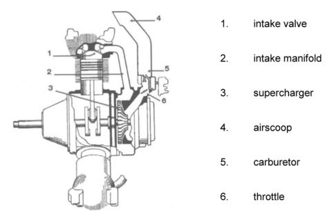
Figure A-3 Supercharger Components
