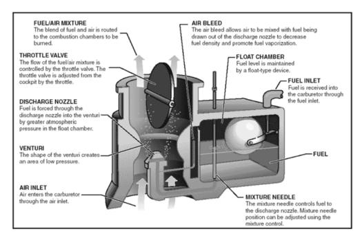
Figure B-1 Float-type Carburetor
