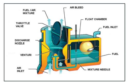
Figure A-5 Float-Type Carburetor
