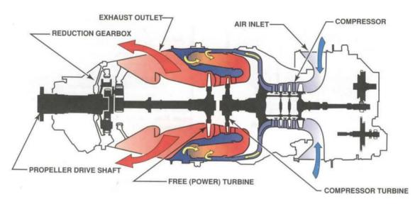
Figure A-4 Free Turbine Turboprop Engine
