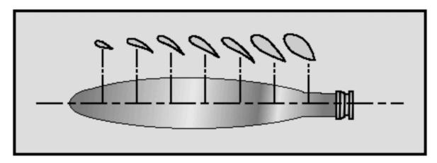
Figure A-1 Propeller Blade Shape
