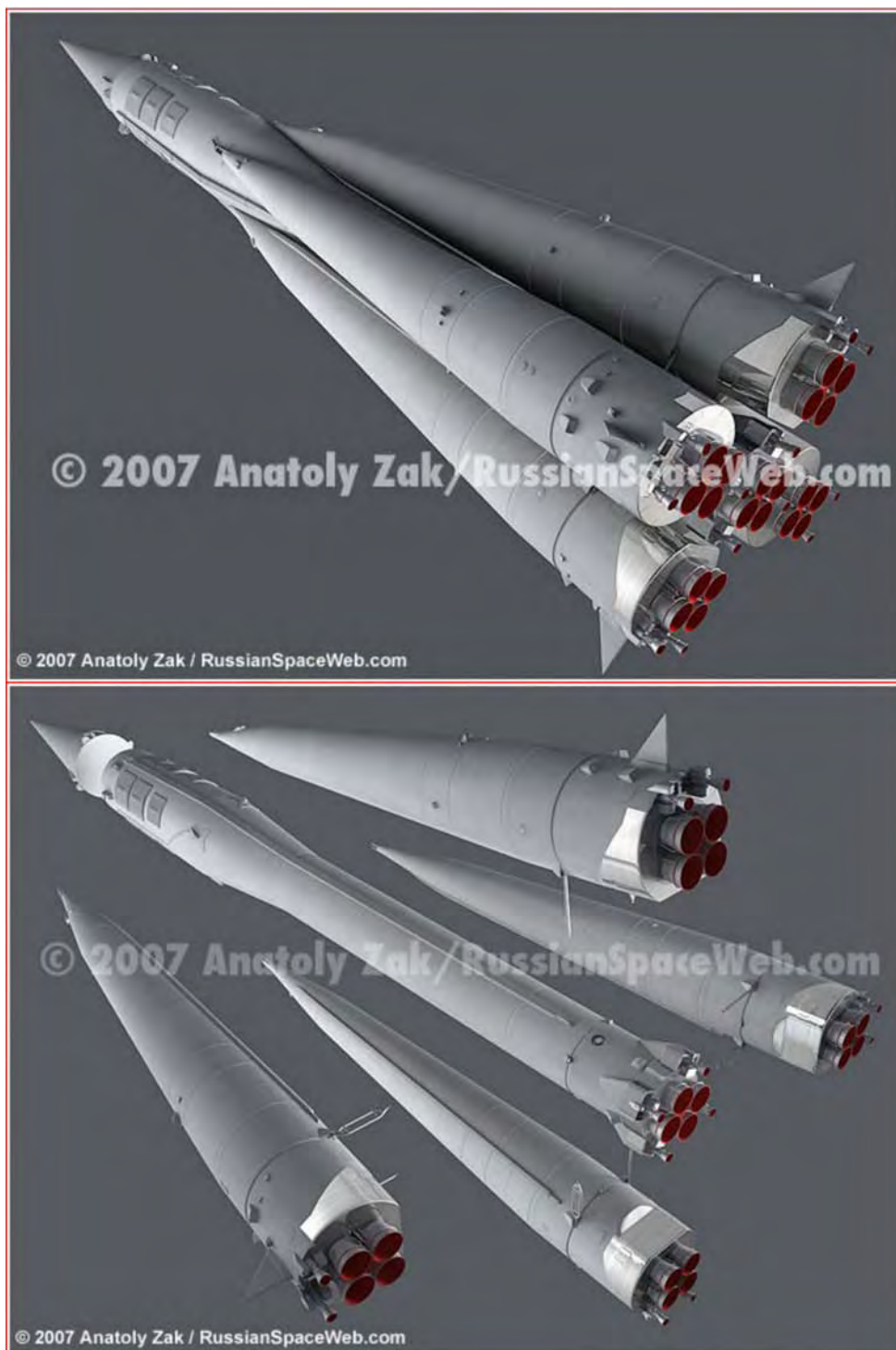
Figure 15P-6 Two-Stage R-7 Rocket Modified for Sputnik-1
